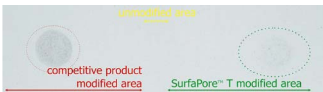
Fig. 9 – Staining performance after steam injection for 2 hours, using a xylene based black marker. The image depicts efficiency after ageing and washing the sample.
