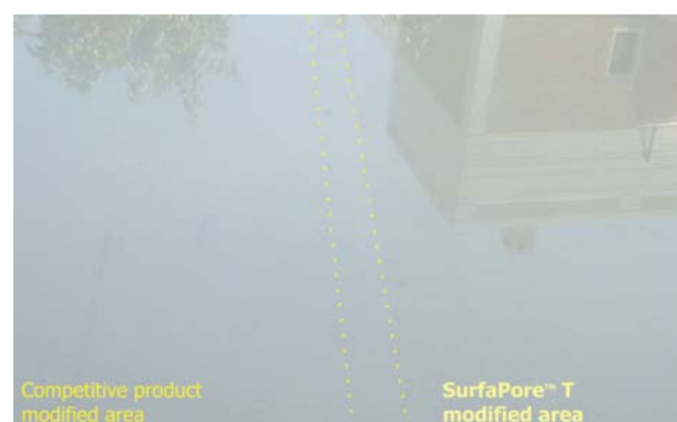
Fig. 4 – Picture of a modified, white porcelain stoneware tile after stain-proofing treatment. Both SurfaPore™ T and competing areas are depicted. The middle stripe indicates a non-modified area.
